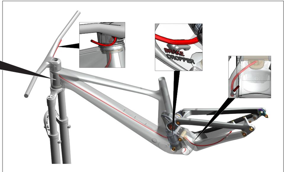
**297134 SCO CABLE GUIDE H-TUBE INNER SCALE AL 23**
